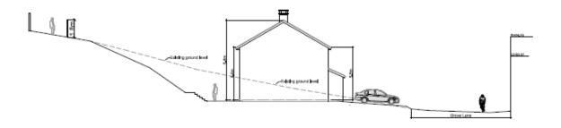
The dotted line on the cross section above indicates the existing ground level which would be excavated to provide level ground for the proposed terrace.
