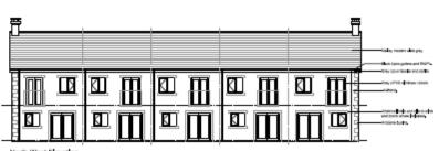
North West Elevation 1;100 Scale The front and gable side facing Cliff Street would be constructed in coursed stone whilst the gable adjacent to the neighbouring property at no. 1 Grove Lane would be rendered.
